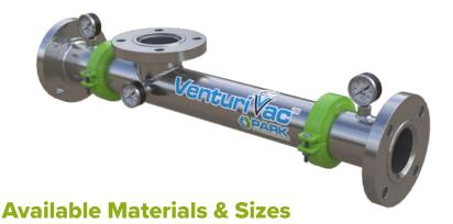
Park Process VenturiVac™ eductors are available in a variety of materials of construction. The eductor is comprised of a main body with a nozzle and diffuser insert. The eductor body is made of carbon steel, stainless steel, PVC or other customer specified material. The nozzle and diffuser inserts are typically made of a chemical and abrasion resistant material such as ultra-high molecular weight polyethylene (UHMW) or Teflon.
