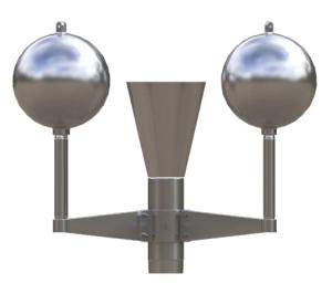
The SkimPro<sup>™</sup> Model D employs a specially designed suction head to pass the engineered required flow rate for water skimming applications. The floats are sized to accommodate the overall weight of the skimmer. Suction heads are equipped with vortex breakers to prohibit air from entering the water flow. The SkimPro<sup>™</sup> Model D can be designed to skim water at flow rates from 25 to over 1,000 gpm.
